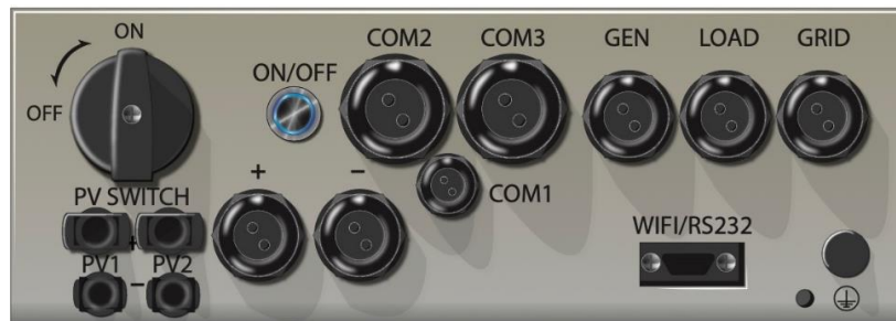
Figure 28 - 3.6kW/5.5kW bottom view.
